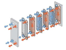
Flow principle of a plate heat exchanger
