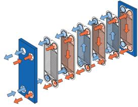
Flow principle of a plate heat exchanger
