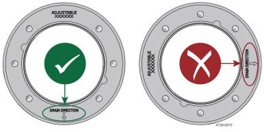
Figure 2: Draining direction
