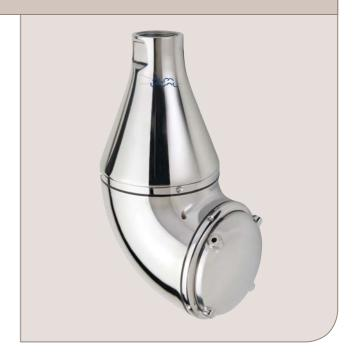
In the first cycle, the nozzles lay out a course pattern on the tank surface. The subsequent cycles gradually make the pattern denser until at full cleaning pattern is reached. Once the full cleaning pattern is reached, the machine will start over again and continue to perform the next full cleaning pattern.
