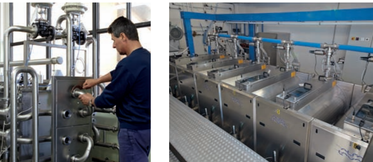
Express heater for low temperature extraction (left) and energy saving round Atmosphera malaxers (right)
