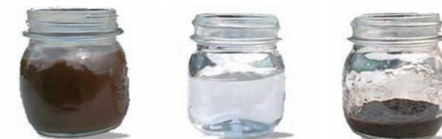
Black water (left) separated by BlueVap into clear water (middle) and concentrate (right)
