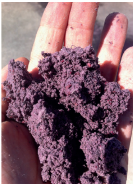
Samples of liquid and solids outlet after separation with Foodec decanter
