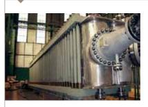
The Alfa Laval Packinox weighs up to 350 tonnes, and one is usually enough to handle the required length of the thermal storage system.
